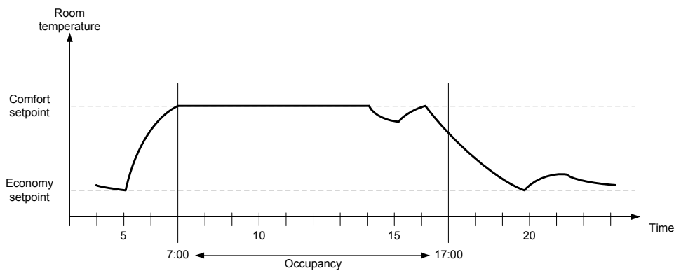
Fig. 10 Room temperature curve for Switch-on/switch-off compensation
