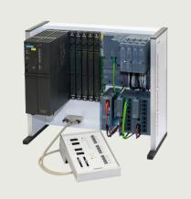
The DCS Digital Base Unit V2.0 training system with CPU 410-5H is used to provide practical training in the configuration of a SIMATIC PCS 7 or SIMATIC PCS neo process control system using a real CPU 410-5H controller.
