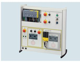
The training case is used realistically practice the programming, operating and commissioning of failsafe SIMATIC S7-1500 controllers within TIA Portal.
