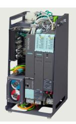
The training case is used to practice and demonstrate the programming, operating and diagnostics of SINUMERIK 840D sl with the drive system SINAMICS S120.
