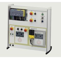
The training case is used to realistically practice the programming, operating and commissioning of failsafe SIMATIC S7-1500 controllers within TIA Portal.
