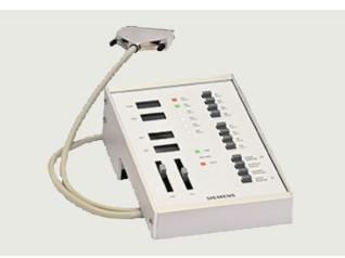
The DCS Digital Signal box is used to provide practical training in the configuration of process control systems SIMATIC PCS 7 or SIMATIC PCS neo using the integration of process signals.
