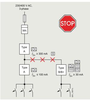
It is not permitted to branch electrical circuits with these types of electrical loads after pulse-current-sensitive residual current protective devices (type A).
