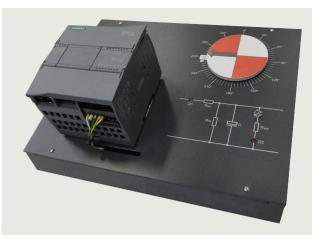
The training module is used to work with the Technology Functions (Motion Control Axis and PID Loop Control) of the SIMATIC S7-1200 in realistically practice exercises. It serves as an extension of the SIMATIC S7-1200 and SIMATIC S7-1500 training devices.
