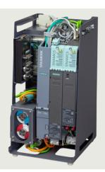
The training case is used to practice and demonstrate the programming, operating and diagnostics of SINAMICS S120 with control unit CU320-2.
