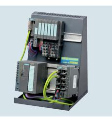
The training case is used to demonstrate and to practice PROFINET within Totally Integrated Automation.
