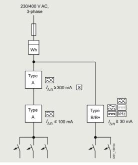
When configuring and installing electrical installations, electrical loads that can generate smooth DC residual currents in the event of a fault must be assigned a separate electrical circuit with a universal current-sensitive residual current protective device (type B) (see configuration example).
