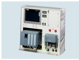
The training case is used to realistically practice the programming, operating and commissioning of SIMATIC S7-1500 controllers within TIA Portal.
