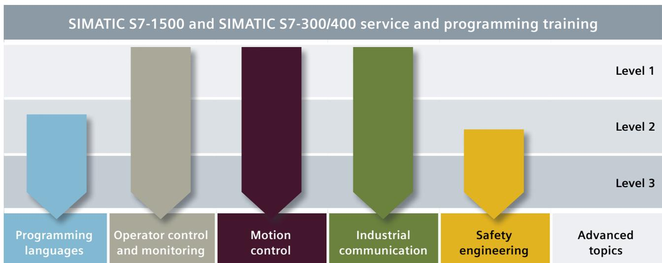
Levels 1–3: Diagram of the 3-stage service and programming training. The programming languages, operator control and monitoring systems, motion control, industrial communication and safety engineering advanced training topics are trained in the depth appropriate for the level.
